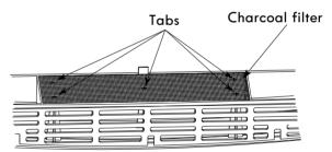
5. Reinstall the vent by sliding the bottom of the vent into place. Push the vent top into position and slide right into place. Replace the two vent mounting screws located on top of the microwave using a #1 Phillips screwdriver.
